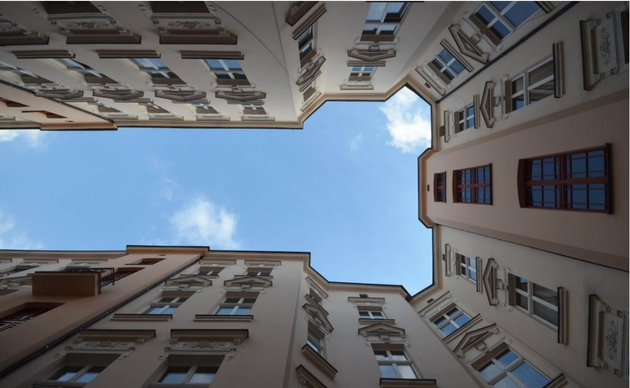
Typical courtyard plan as seen when looking from the bottom of a courtyard, up. Niches on corners allow additional light and air into corner apartments
